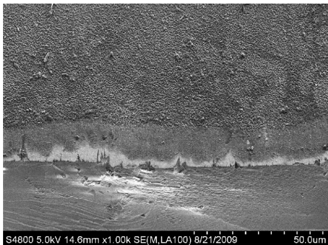
Fig. 18. The cross section of the Al NRs on Cu substrate after 100 cycles (10,000 \times ).
